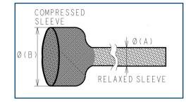
Diameter is measured over a mandrel. Length for cut pieces is measured in a relaxed position.
